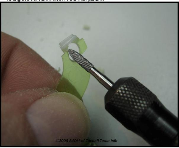
9. Drill 2 holes for the wires at the feet of the fibre optics.
