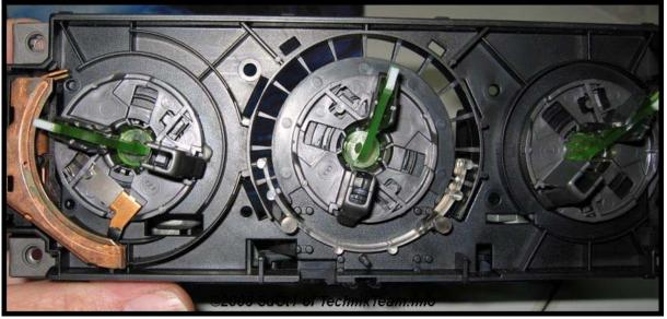
6. This photo is from the Golf MK III HVAC. The fibre optics of the knobs at the Corrado looks a little bit different. The outer two are not green. The optics in the middle is the fibre optic for the knob and the bulb holder. Press the bulb holder and pull them out. Pull out the bulb, they is no longer needed.
